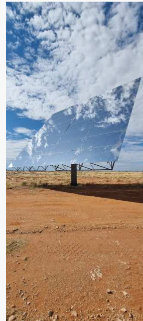
□ Heliostat built with the new facets manufactured by Abengoa.
