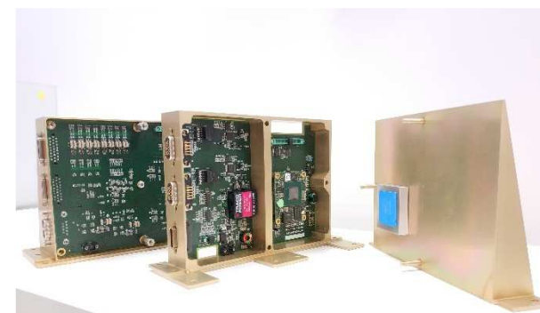
□ Interior view of the electronic modules of the Battery Diagnosis Unit (BDU).
