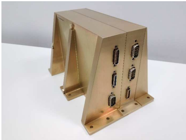
□ Engineering model of the Battery Balancing and Diagnostic Module (BDU).
