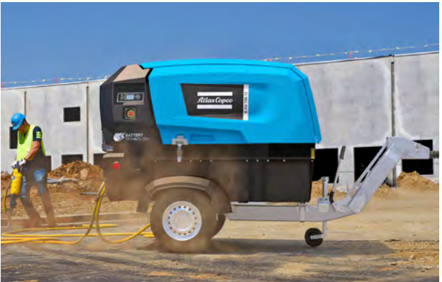
The world's first battery powered screw compressor, B-Air, launched in 2023.
