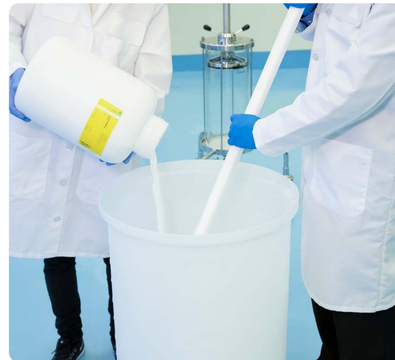
Preparing CHT resin slurry in container for column packing
