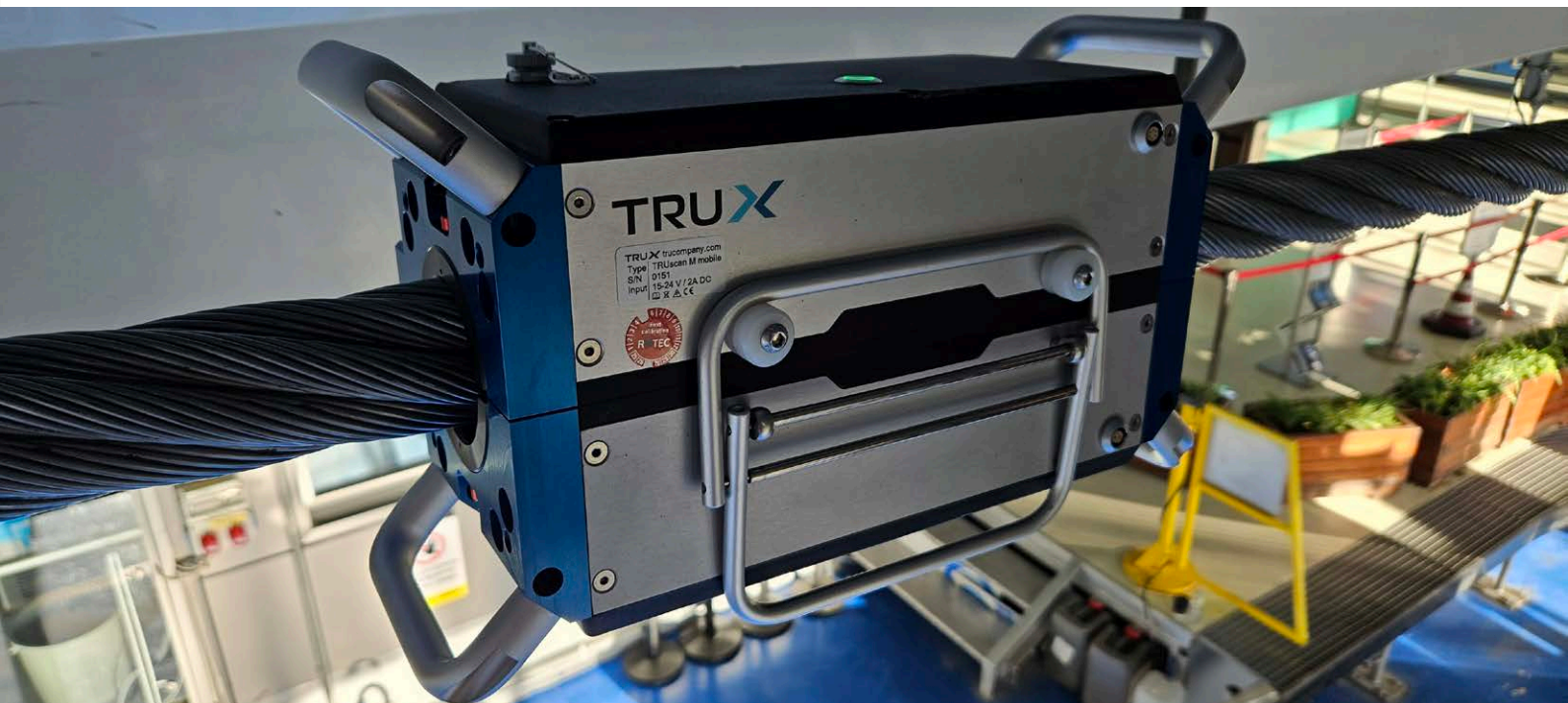
TRUscan on a cable car in Bursa (Turkey) – for reliable and data-based rope management.
