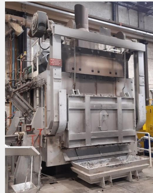
> A reverberatory melting furnace at C-TEC, Constellium's R&D center in France
