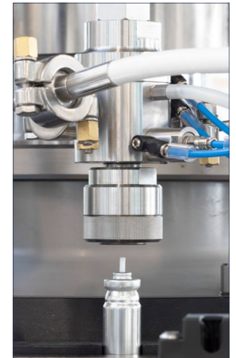
1 st green gas filling machine for pMDIs for new generation green propellants (HFA 152a & HFO 1234ze)
