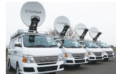
Portable mobile base stations
