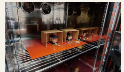
Charge-discharge cycle tests in simulated stratospheric conditions
