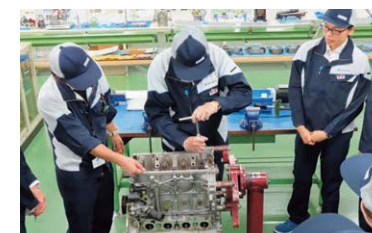
Practicing the assembly of automotive engine bearings
