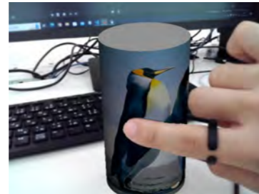
Touching a tangible object onto which the image of a bird has been superimposed in the AR space. The tactile sample developed by DIC allows the reproduction of a highly realistic texture. (This photograph was taken at Saitama University's Komuro Laboratory.)
