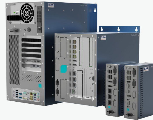
ProSys Embedded computing platform. Industrial applications Systems © Elma
