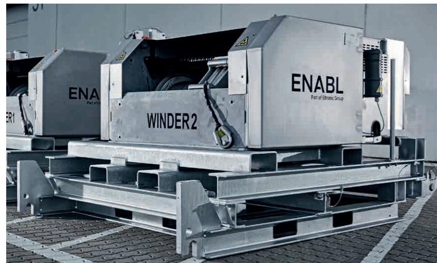
ENABL A/S Tagline Master System on Ground Frames
