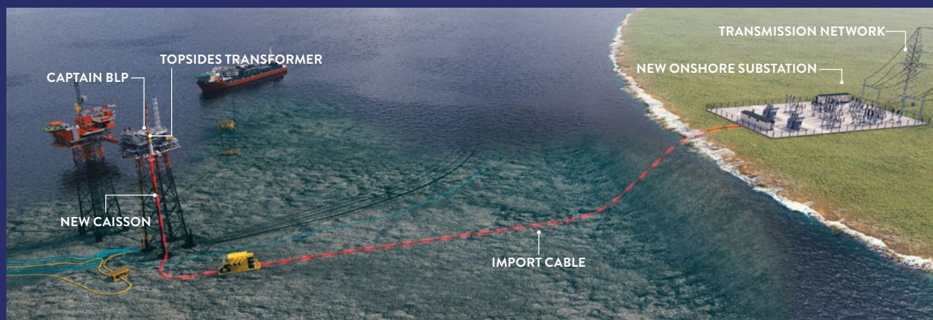
Fig – FEED graphic of potential Captain electrification option showing shore tie-in and new subsea cable, caisson and topsides equipment.
