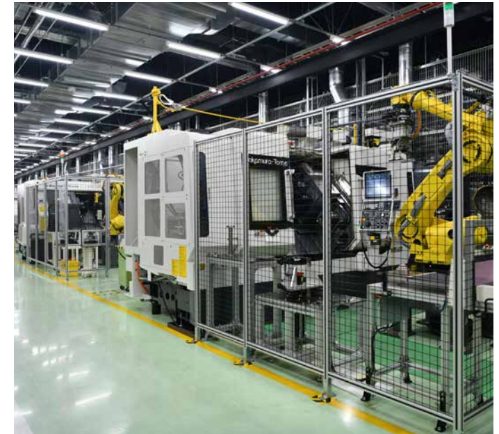
Machining cells connected to an automatic warehouse
