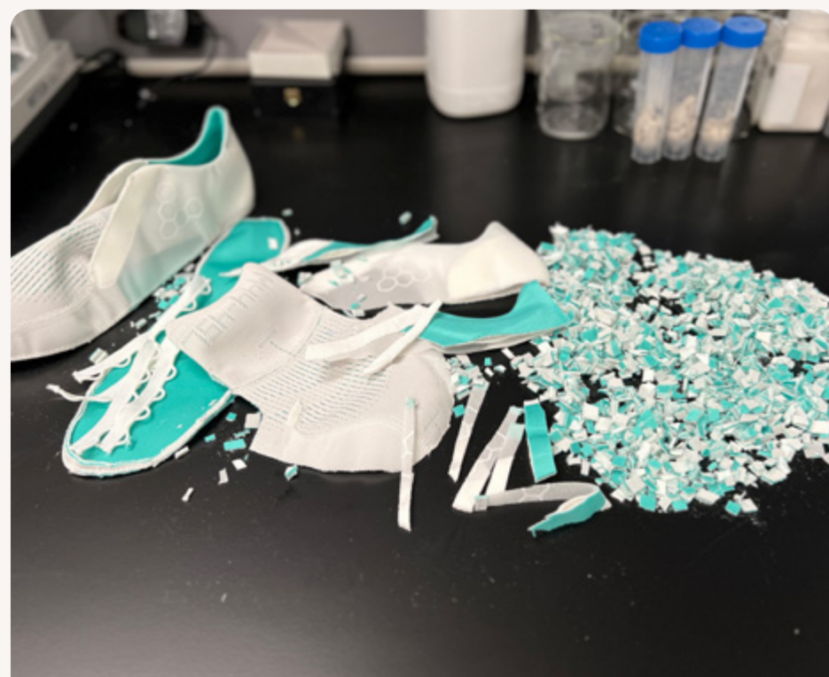
A disassembled Primus ready for chemical recycling by Circ
