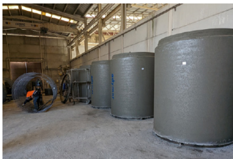
Prefabricated elements for sewerage pipelines of mixed sections, deployed on the sewerage and wastewater treatment works in Montijo-Puebla de la Calzada (Badajoz)
