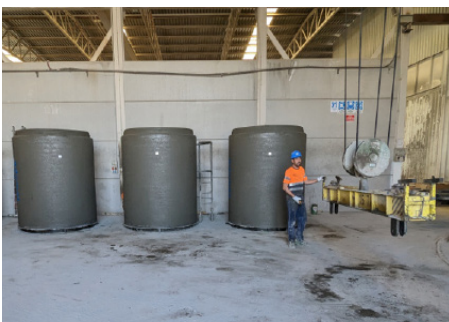
Prefabricated elements for sewerage pipelines of mixed sections, deployed on the sewerage and wastewater treatment works in Montijo-Puebla de la Calzada (Badajoz)
