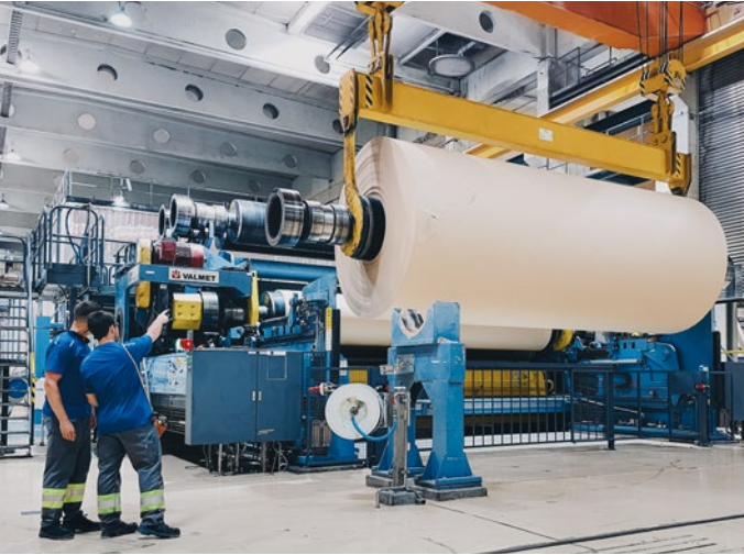
↑ A tambour with unbleached kraft paper on the newly converted PM6 in Steyrermühl
