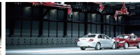
Indoor omnidirectional crash test facility
