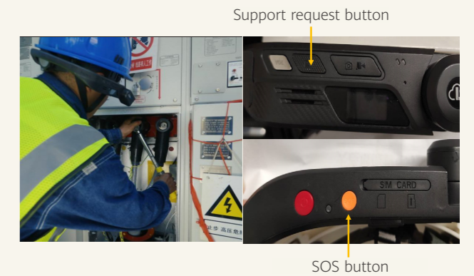
Delivery: A smart safety helmet requests support and sounds alarms, while a cloud platform provides real-time feedback.
