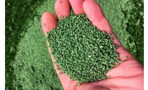
PRO-gran crumb rubber made by casing tyres
