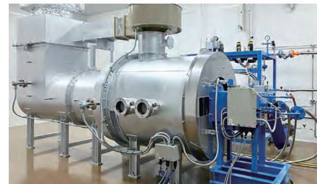
Hydrogen mixed combustion burner available for customer demonstration at the Iwatani R&D Center
