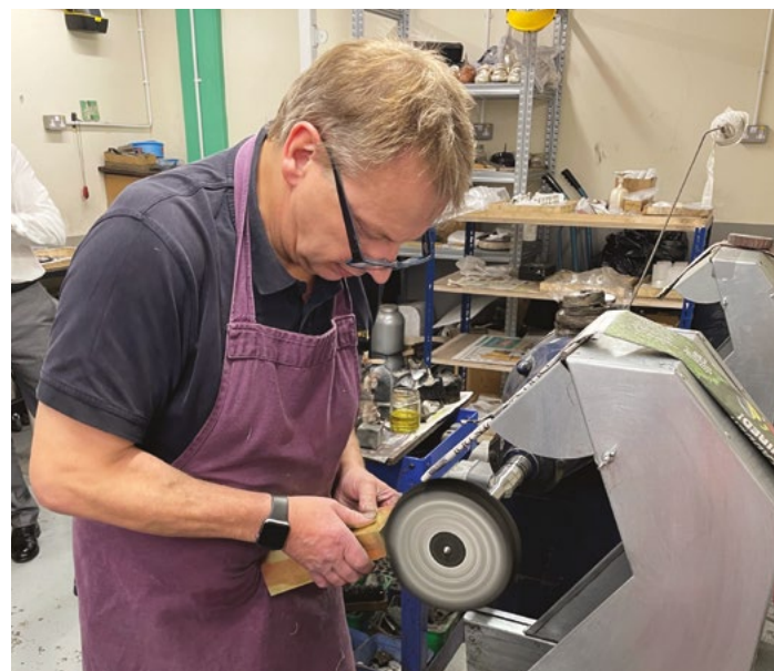
Fine particles of silver generated by our Silver Workshop are filtered at source and collected for recycling by our precious metal supplier. Each year, we recover up to 10kg of silver using this method.
