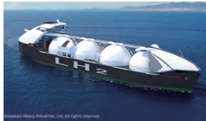
Concept image of a 160,000 m³ liquefied hydrogen carrier Photograph provided by Kawasaki Heavy Industries, Ltd.
