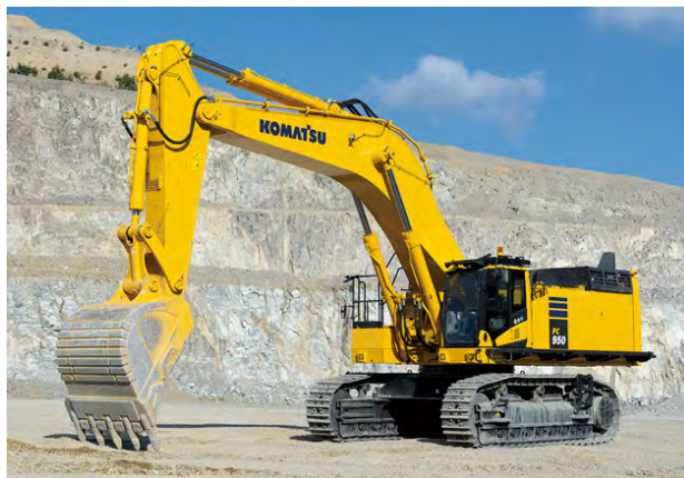
PC950-11 with the “KomVision” bird’s-eye-view camera system as a standard feature.
