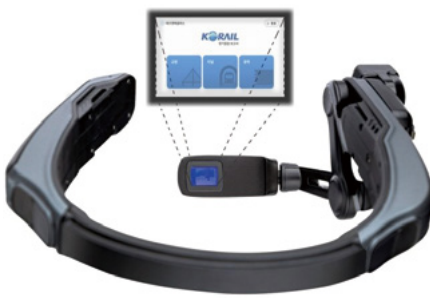
Voice Recognition Based Smart Glass for Inspection on Railroad Facilities
