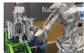
Robot replacing refractories for molten steel flow control
