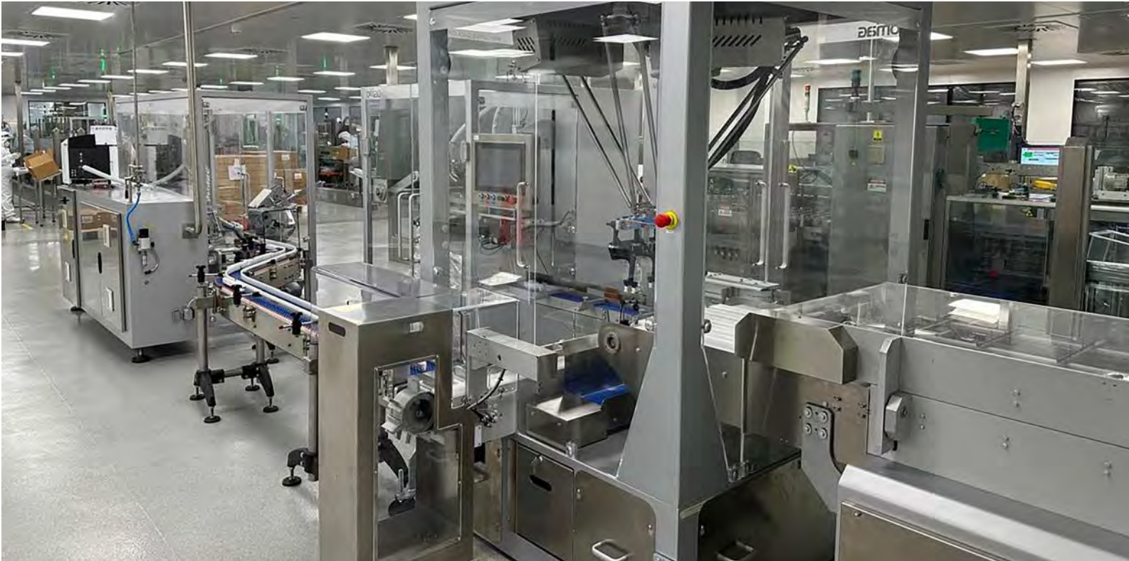
From four machines to one: Our cutting-edge stick pack machine in our Santiago site streamlines the entire production process for single-dose sachets
