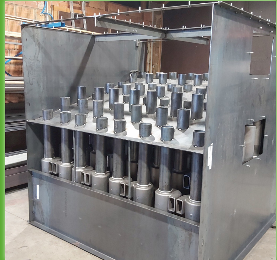
Above: The heart of the process - the multicyclone battery.
