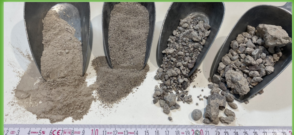
Above: S/CRETE materials (from left to right): Cement stone, sand, aggregates, crushed concrete.
