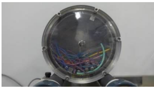
▲Separation of coating materials swollen by an organic solvent
