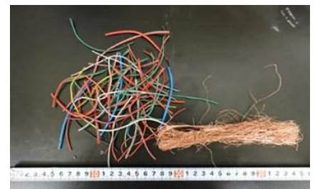
▲Copper wires and coating materials after separation by the combined plastic swelling and ball milling method
