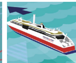
The pressure difference causes a lift (thrust) force perpendicular to the wind direction.
