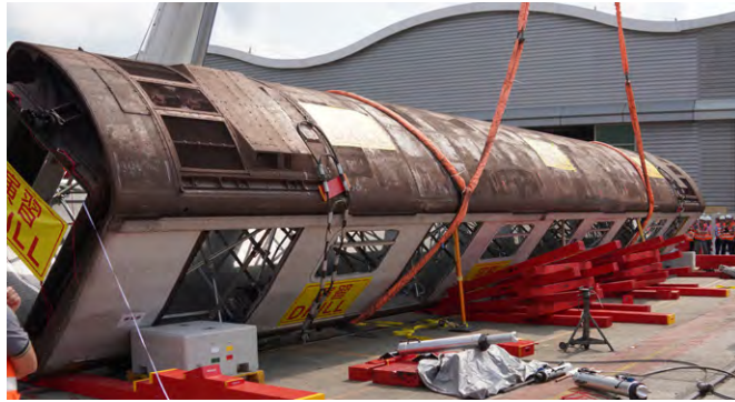
Uprighting process of a toppled M-train trailer car
