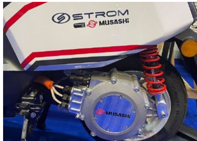
STROM prototype vehicle equipped with Musashi EV drive unit
