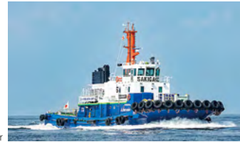
Sakigake, ammonia-fueled tugboat converted from LNG-fueled predecessor
