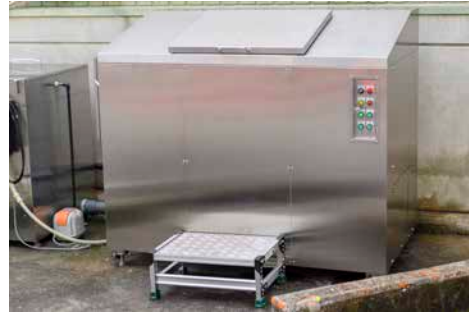
Introduced food waste disposal machines that harness the power of microorganisms
