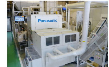
Near-infrared sorting machine that can sort three types of resin simultaneously
