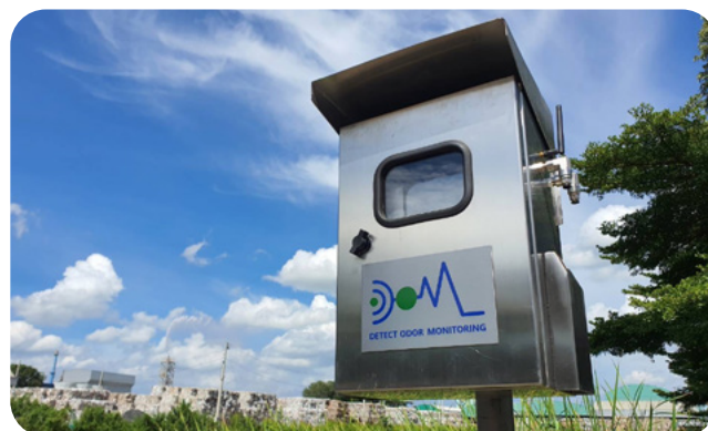
E-Nose or D.O.M (Detect Odor & Monitoring).
