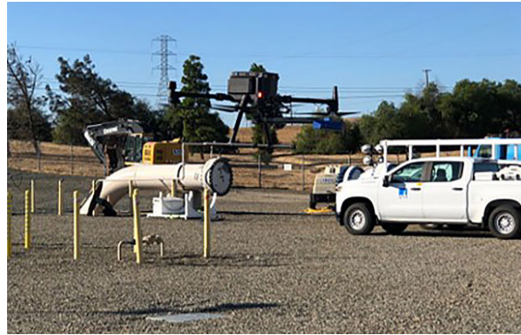
PG&E is piloting the use of drones to identify methane emissions at compressor stations and storage facilities.
