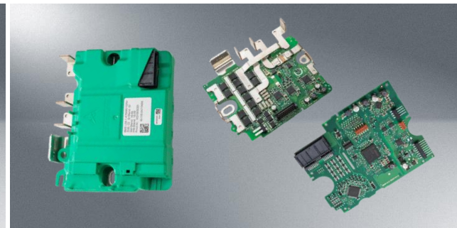
Battery Management Control Units
