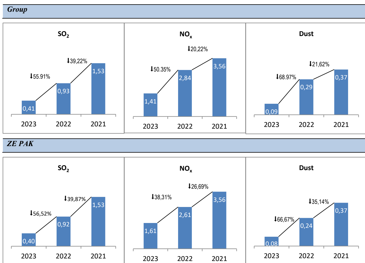
Graph 22: Total SO 2 , NO x and dust emissions to the atmosphere (thousand tonnes)
