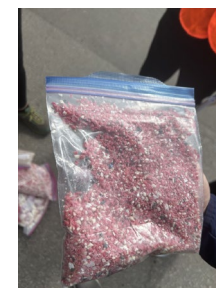
Flakes from the tubs, made of PUR & PE.
