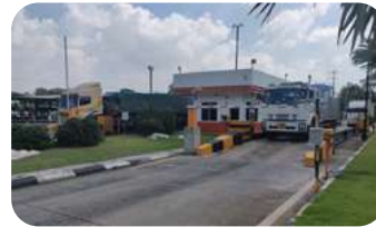
Automated truck scale systems to minimize manual labor and improve transparency in the weighing process, Siam Kraft Industry Co., Ltd.
