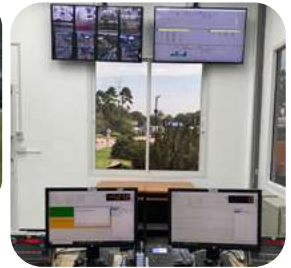
Automated truck scale systems to minimize manual labor and improve transparency in the weighing process, Siam Kraft Industry Co., Ltd.
