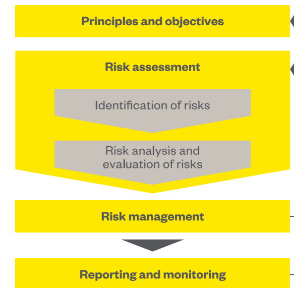
General risk management process (in accordance with the International Organization for Standardization: Risk management. Instructions)
