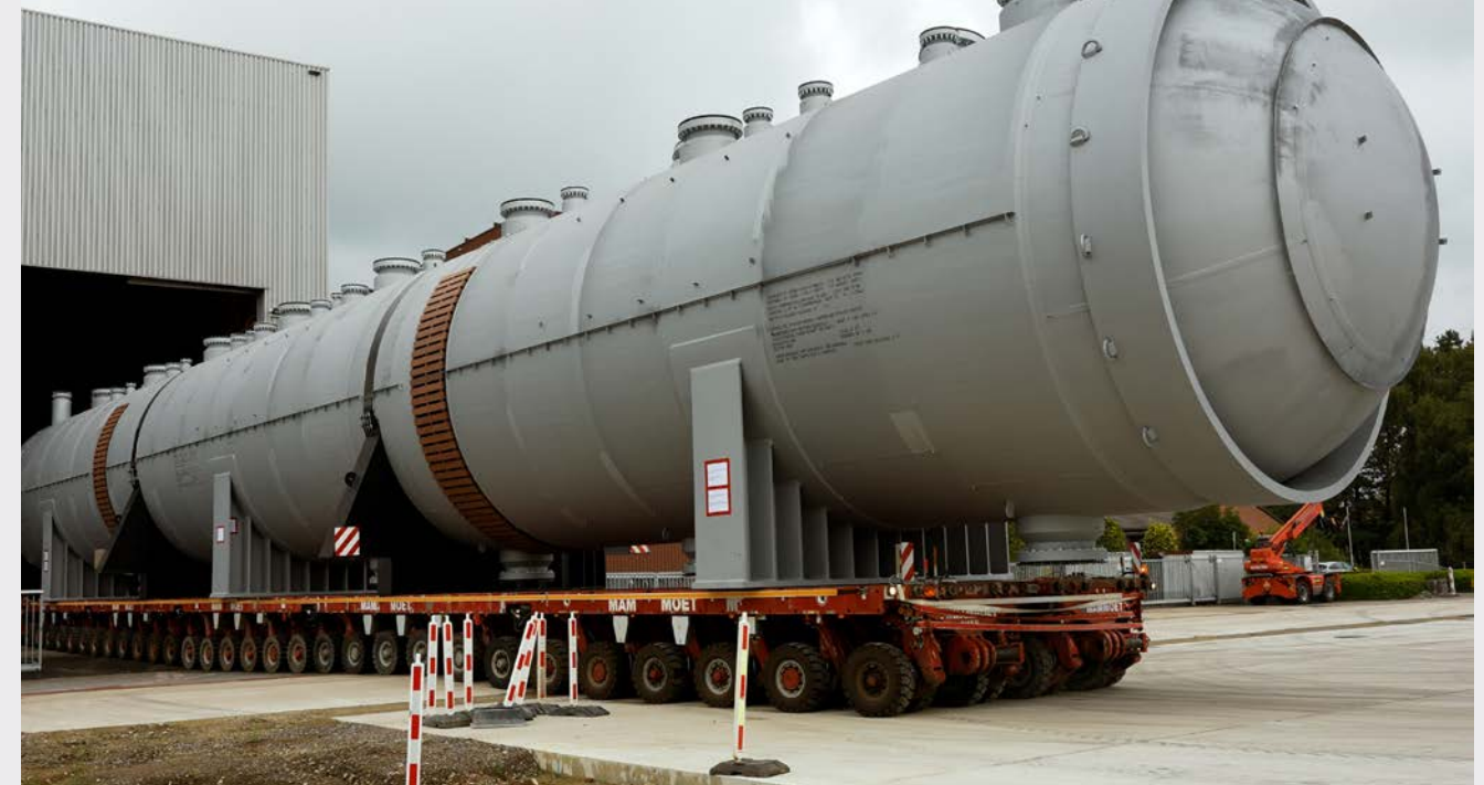
The autoclave Weight – 1,100 tons, length – 50 m, diameter – 6 m
