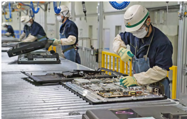
TV being dismantled at Green Cycle Corporation
