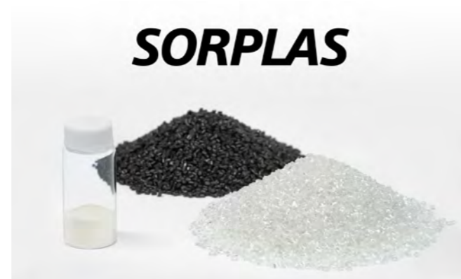
SORPLAS recycled plastic pellets (black), recovered pellets (transparent: right) and Sony's original flame retardant (left)
