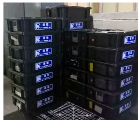
Returnable container used to transport components at Sony Global Manufacturing & Operations Corporation
