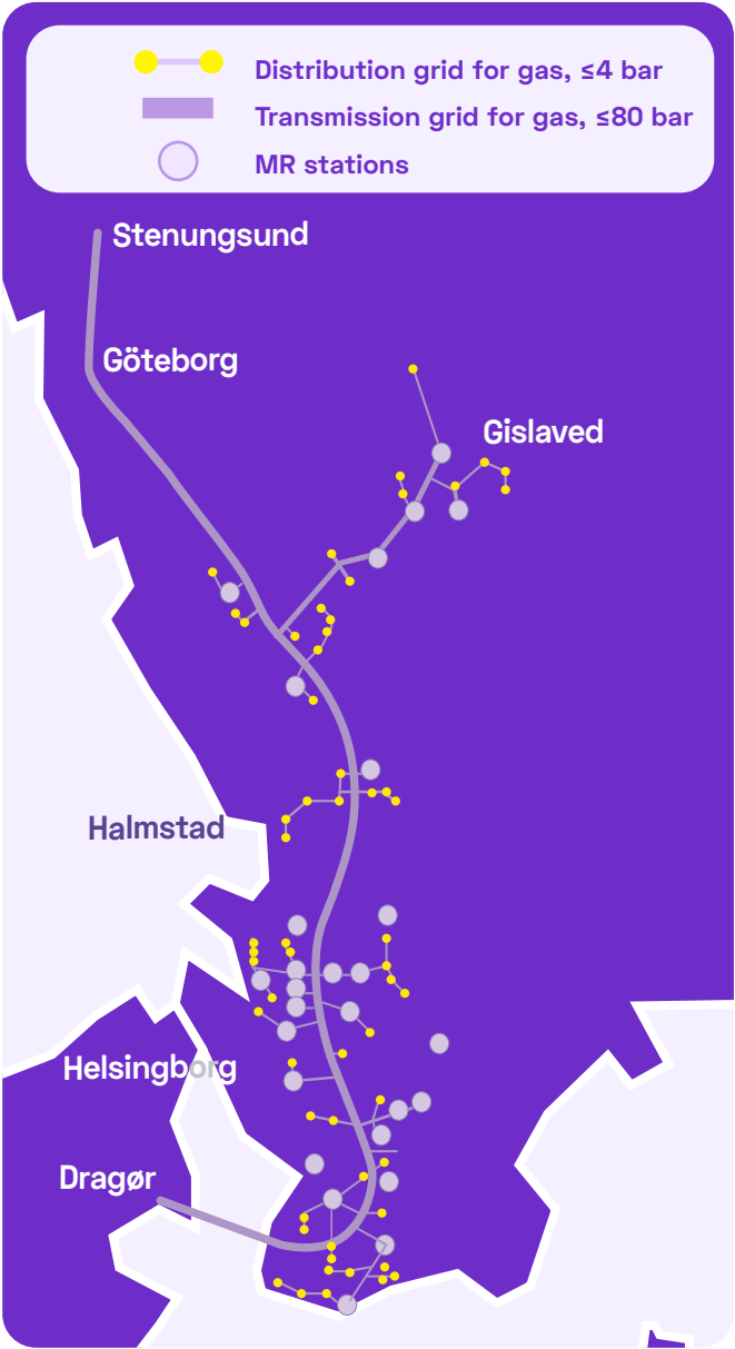
Gas network in southwestern Sweden
