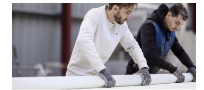
Manufacture of composite poles
