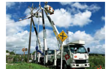
Original Pole Replacement Vehicle Developed by TEPCO PG This patent is licensed to other companies and widely utilized.
