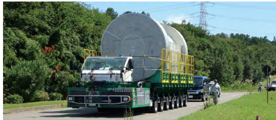
Transport of Spent Fuel from Kashiwazaki-Kariwa Nuclear Power Station to Interim Storage Facility
