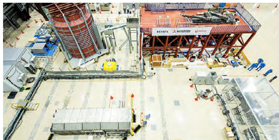
Mock-up of Fukushima Daiichi Unit 2 at JAEA (Upper Left) and Robot Arm (Upper Right)
