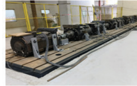
8 Traction Motor Set up for System Test
