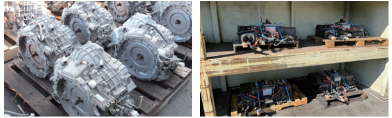
Recovered end-of-life HEV motors Recovered end-of-life FC stacks
