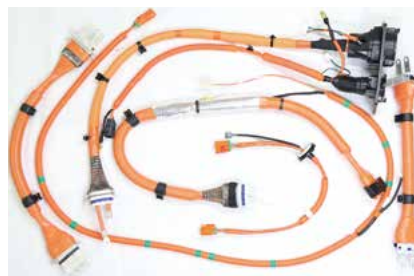
High voltage wire harnesses
